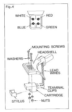
When you have connected signal wires, install cartridge to the head shell as shown in Fig.4. Do not fully tighten screws. Replace stylus in the cartridge.
